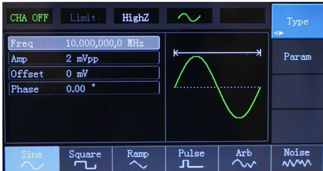
Single Channel, Multiple basic waveform options
